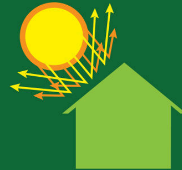
Reflective and Emissive Cool Roof Surface
